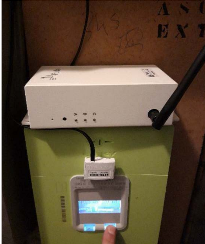
Pulse sensor for Linky smart meter
