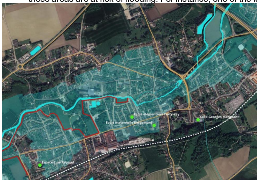
Figure 9: Extent of the water pocket on the city of Blendecques during the January 2024 flood. The red lines represent the dykes that had been put in place after a 2002 flood episode.
